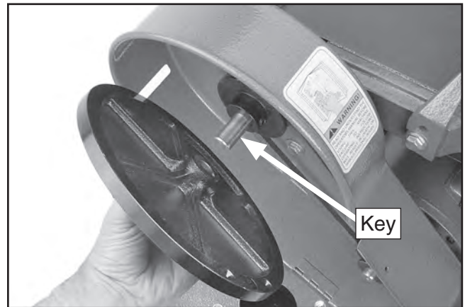
Figure 27. Installing plate onto drive shaft.
